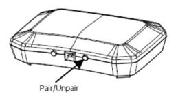
The 2-pin connector on the sensor module allow for the small round sensors to be utilized. Extra sensors XS-02 can be used to build a nest of hard-wired sensors that all report to one sensor module.
