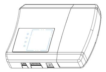
The 6-pin connector provides the wire to the valve(s) and to the hard-wired sensor. Multiple hard-wired sensors can be connected in daisy-chain from the controller directly.
